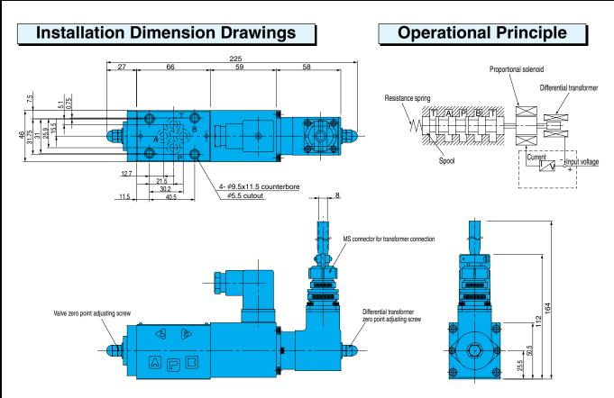
The gasket mounting method conforms to ISO4401-AB-03-4-A.
